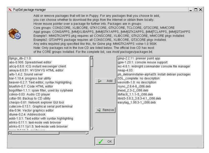
On the left side you can see all programs available. On the right side you see the programs already installed. Mark in the right list the program, which you would like to deinstall. Click on the button "Remove" between the two lists. Afterwards you press the button "OK".
