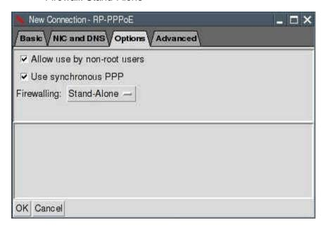
Afterwards press the "OK" button. A new window appears "RP-PPPoE". There are two buttons named "Start" and "Stop".
