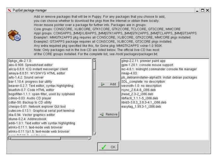
On the left side you can see all available programs. On the right side are the PupGet programs already installed (at the beginning this list is empty). Now select in the left list the program which should be installed and click on the button "Add" between the two lists. This transfers the program into the right list. Then you click on the "OK" button and the program will be installed.
